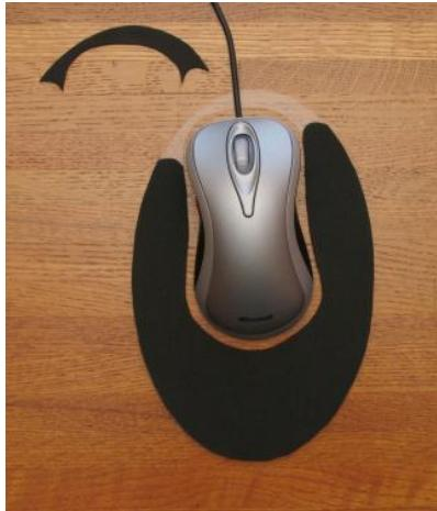
Alternate modification would be to cut the foam and plastic for more vertical movement
